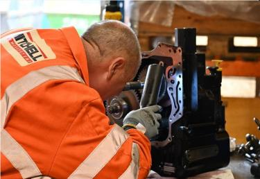
The transmission reassembly processes include using remanufactured/rebuilt parts and components and new wear parts (gaskets, seals, bolts, screws, etc.) All new parts used are always Dana Spicer® Genuine Parts.
